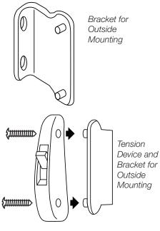
Outside Mount: Align the mounting bracket screw holes with the pencil marks. If mounting into wood, predrill screw holes and then install the mounting bracket using the 1" Phillips head screws provided.
