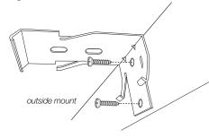
**Step 4.** Securing the Head Rail Position the head rail so that the ridge on the top-front of the head rail fits into the front of the bracket as illustrated, and then push upward until the metal tabs on the back of the bracket snap onto the back of the head rail.
